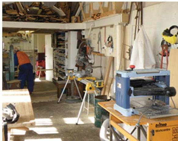
*Figure 62 – Thicknesser and mitre saw*
