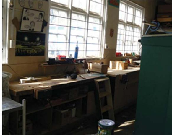
*Figure 61 – Workbenches utilising natural light and away from main throughfares*
