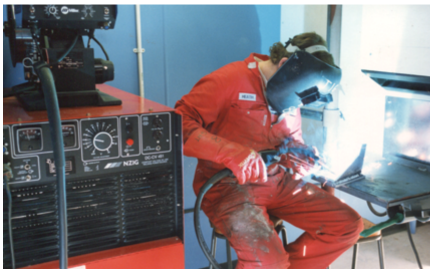
A student demonstrates metallic inert gas (mig) welding during a polytechnic engineering course. Otago Polytechnic
