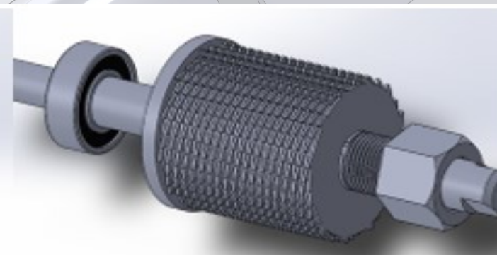
Figure 3a, 50 discs are sandwiched
