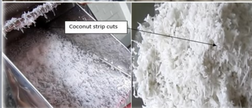
Figure 7 New design cuts (top), original shredder cuts with strips (bottom)
