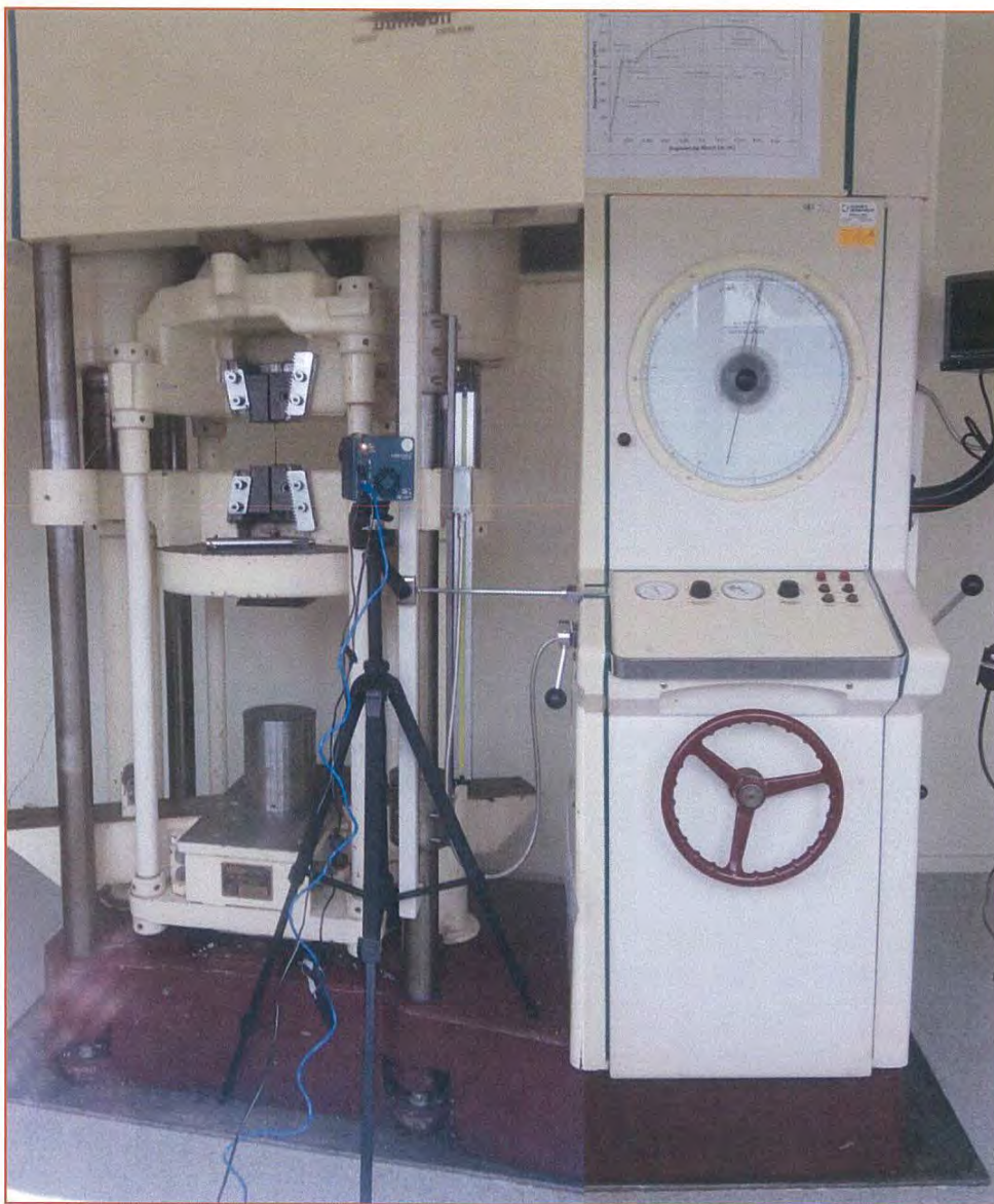
Figure 3-3: Dennison Universal testing machine used for mechanical loading of specimens
