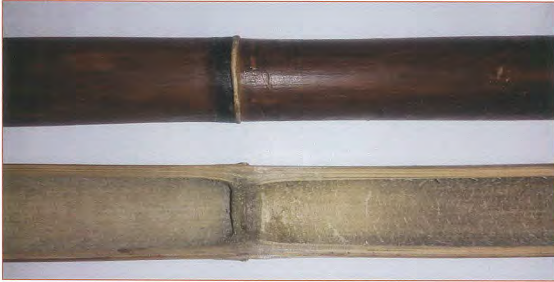
Figure 3-1: Bamboo Himalayacalamus hookerianus specimen split in half exposing node boundary and wall cross section (dark colour is due to heat treatment)
