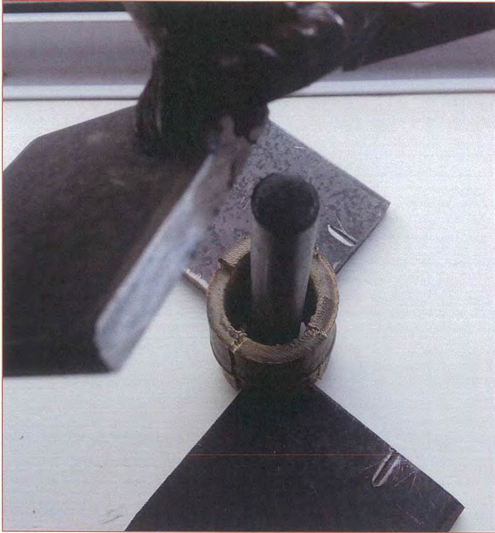
Figure 7-9: Shear failure points visible in specimen after removal of upper section of apparatus
