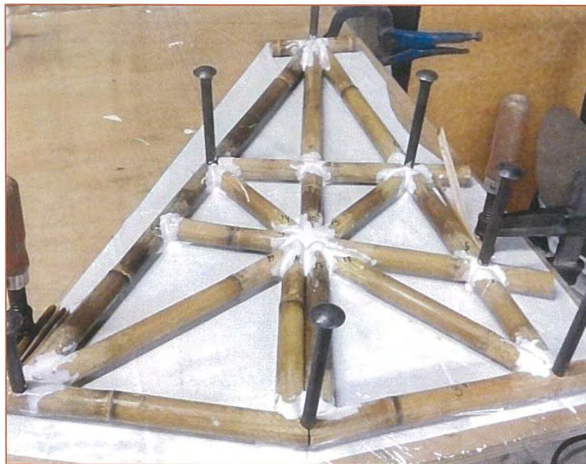
Figure 7-23: Complete frame pinned flat in place, joints tacked together with additive-thickened epoxy resin.
