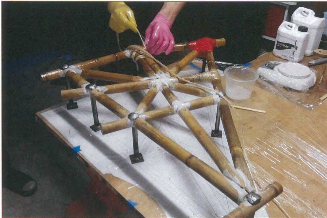
Figure 7-25: Layering joints with impregnated fibre-resin matrix. Frame shown in final position lifted off backing board by fixings.
