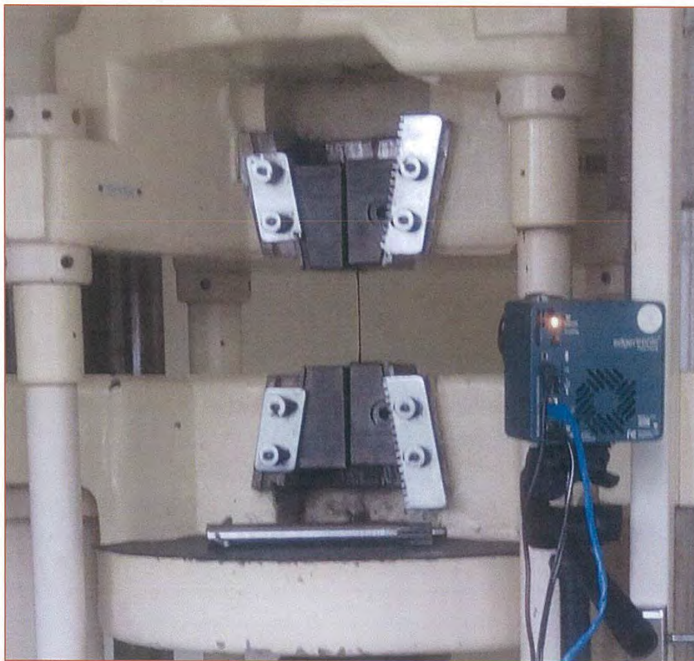
Figure 7-10: Specimen in position between vice-jaws of Dennison testing machine
