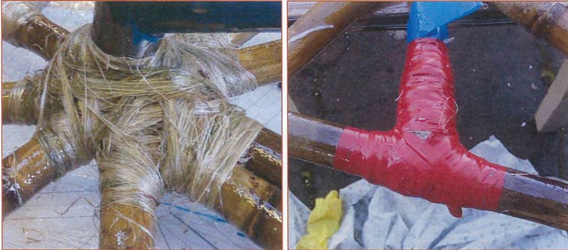
Figure 7-26 Joint wrapping process. Left: Wrapped resin impregnated fibres. Right: Perforated electrical tape used to remove excess resin and compress fibre matrix.
