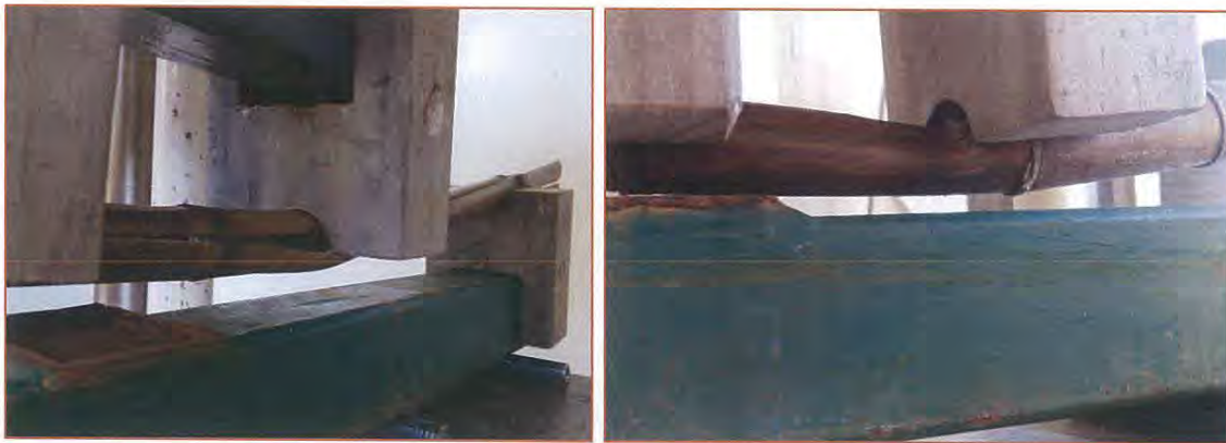
Figure 7-5: Bending failure modes exhibited by specimens. Left (a) longitudinal splitting of culm. Right (b) Crushing of culm wall.
