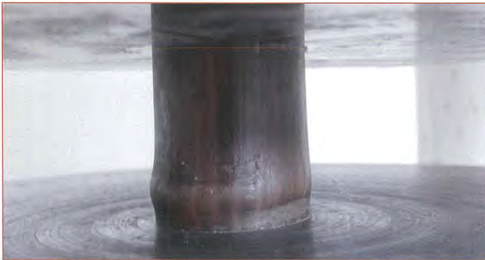
Figure 7-14: Compression loading of specimen showing restriction on radial strain at ends leading to 'barrel' shape developing.
