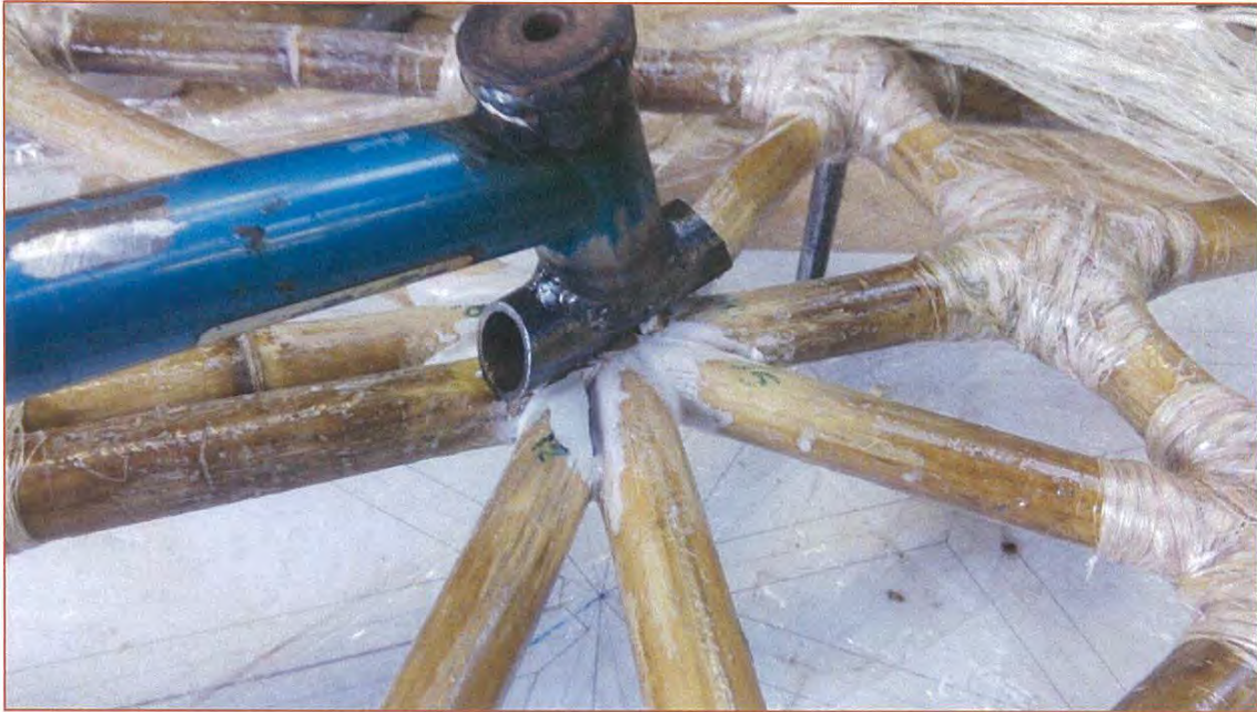
Figure 7-28: Load application point held in position prior to joint wrapping. Note end-piece welded on at 90 degree angle to increase joint rigidity.
