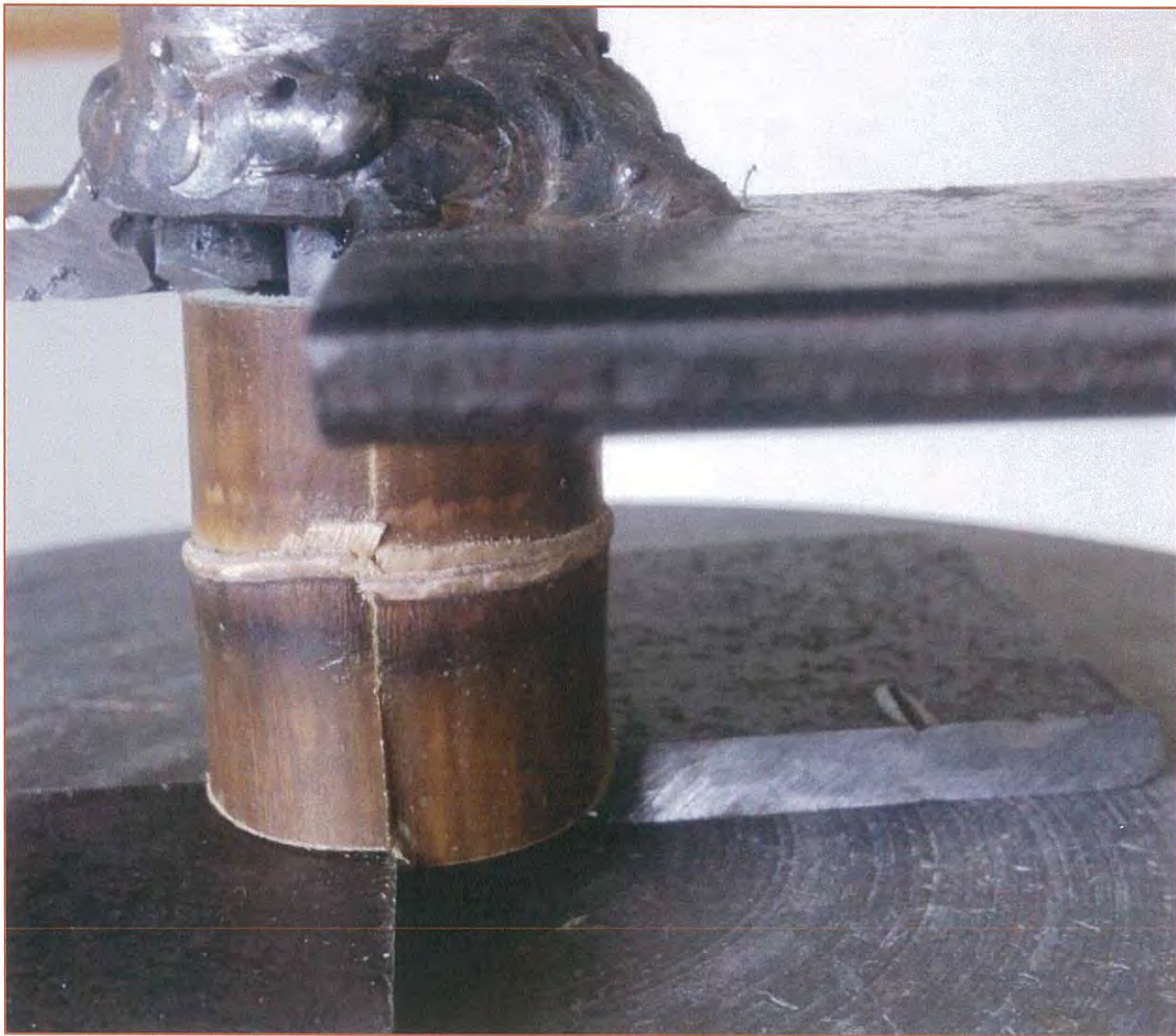
Figure 3-5: Axial shear failure of specimen using testing apparatus
