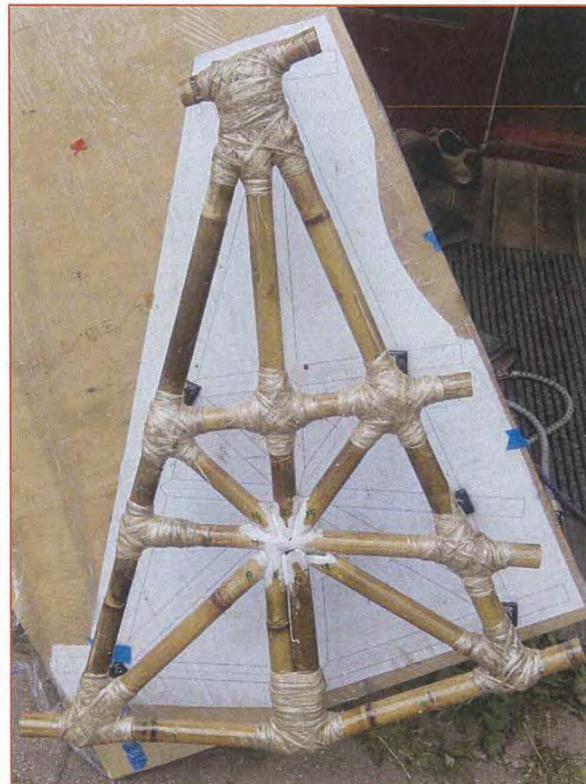
Figure 7-27: Prototype frame with 9 of the 10 joints wrapped and set.
