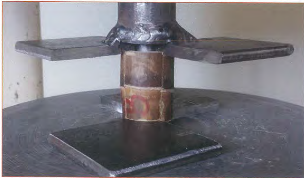
Figure 7-8: Shear lines visible in specimen after continued loading past failure point
