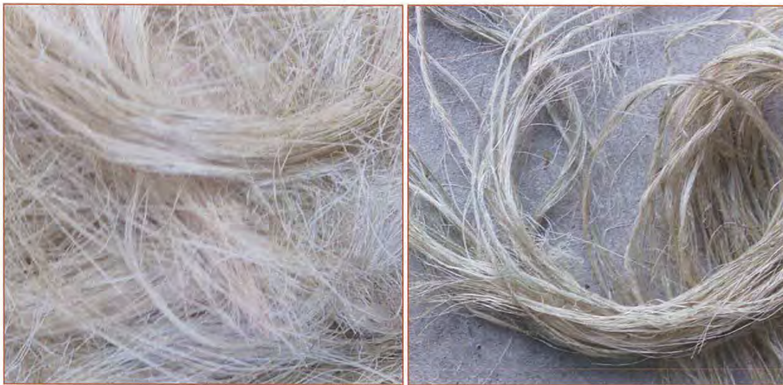
Figure 7-24: Flax fibres used in joint construction. Left: combed loose fibres; right: twisted into loose yarns of approximately 5mm diameter prior to wrapping.
