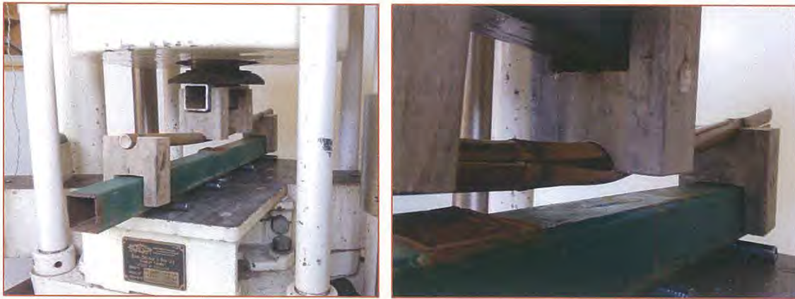
Figure 3-4: Loading and failure of specimen under static four-point bending test.
