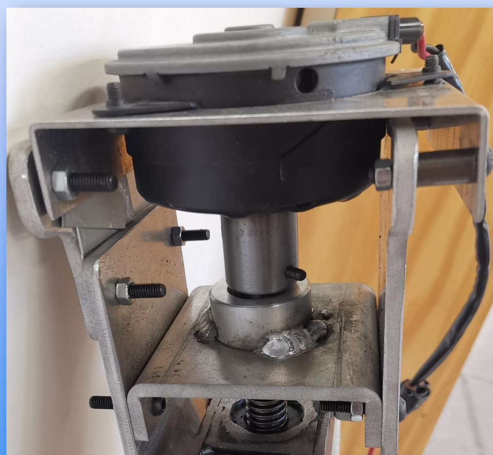
Figure 1—Drive Motor (Runs on 12 V DC)
