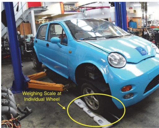
Figure 4 – Gravity force measurement at the individual wheel
