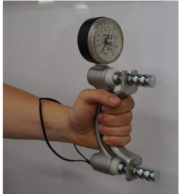
Figure 1-1 Jamar Hydraulic Handheld Dynamometer
